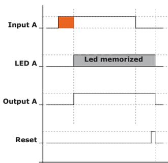
**«Input Memory» or «Automatism»** : The output is activated after filter time delay (when the LED is displayed) and will remain activated so long as the LED will remain visible on the front (the output follows the input memory).
