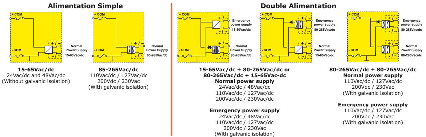
In the case of a model equipped with 2 power supplies, consumption will be via the so-called «normal» power supply, consumption on the «emergency» power supply remaining practically nil. It will only be used in the event of an abnormal voltage drop or failure of the normal power supply. The emergency power supply may consume 10 mA.
