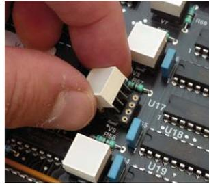
The LEDs are fitted on detachable sockets, enabling a change of colour. The colours available are the following ones :
