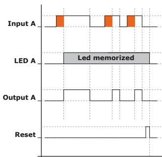
**«Input»** : This function is intended for remote maintenance. It allows a remote operator to know the return to normal and the arrival of a new alarm on an unacknowledged channel and to determine the level of intervention necessary. If the input is still present after the time delay, the output will be activated. If the input is impulsive and disappears, even if the channel is not acknowledged, the output will disappear. It will be reactivated if the input reappears (and after a timeout).
