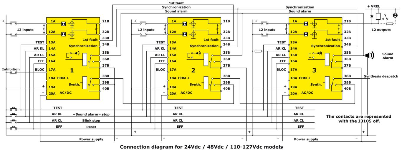
The «+COM» is to be used to power the input contacts. The inputs can be powered directly from the «+» of the J3105 supply voltage (Terminal 19A). **The use of «+Com» is mandatory for the 80-265Vac/dc version.**
